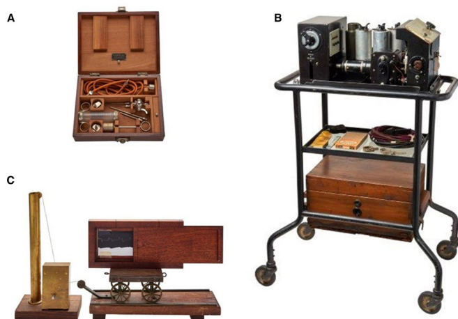
Figure 8 Items from the BCS Museum. (A) Pericardial aspiration kit, 1950, owned and donated by Dr Evan Bedford. (B) Cambridge Instrument Company portable ECG, 1929, donated by Dr Patrick Cadigan. It comprises not only the working parts of the galvanometer and camera but also the trolley, skin electrodes, patient cable, battery case and an unopened box of photographic film. This was the standard ECG in all British hospitals until c.1950 when direct writing machines were introduced. (C) Augustus Waller's model train, track and replica of photographic plate used in recording the first human ECG in 1887.
