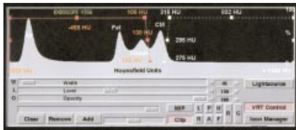
Figure 1 Volume rendering controls with a histogram showing voxel density values. The x axis shows the voxel values, the y axis the frequency distribution. The first peak represents air, the second fat, the third tissue, and the fourth contrast medium (CM). The orange graph represents the range used for visualising vessel, the white graph represents the range used for visualising calcification.
